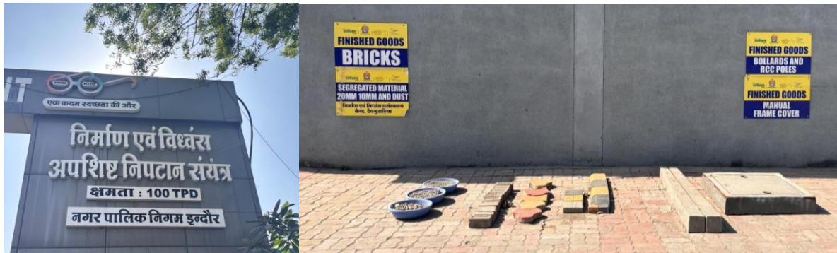
Picture 8: C&D waste processing facility, Indore: Pavement tiles, manhole covers, interlocking tiles etc made from C&D waste are used by IMC
