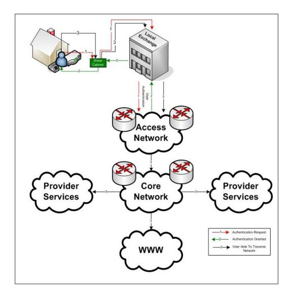
Access Network Connecting the User to the Telecom Service Provider
