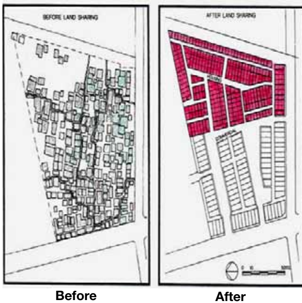
Bangkok: Land sharing through re-blocking, land readjustment, and densification in Baan Manangkhasila Source: CODI.
