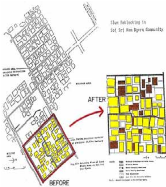
Bangkok: Settlement upgrading through re-blocking, land readjustment, and densification Source: Community Organizations Development Institute (CODI).
